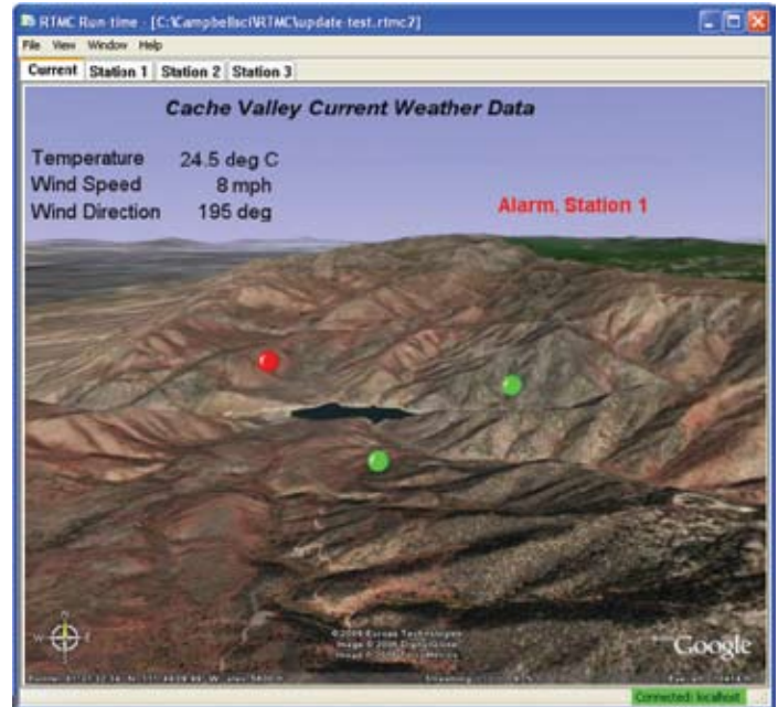
RTMC Pro includes multistate, text, and email alarm capabilities.
