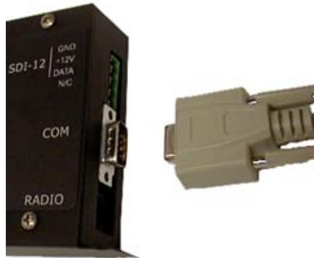
FIGURE 1-3. J5, RS-232C Terminal Interface
