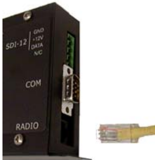
FIGURE 1-2. J6, Radio Interface Port
