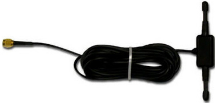
FIGURE 4-4. The surface mount antenna is often used for the base station
