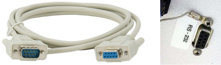
FIGURE 4-2. Serial cable (left) and the weather station serial port in which the serial cable male connector connects
