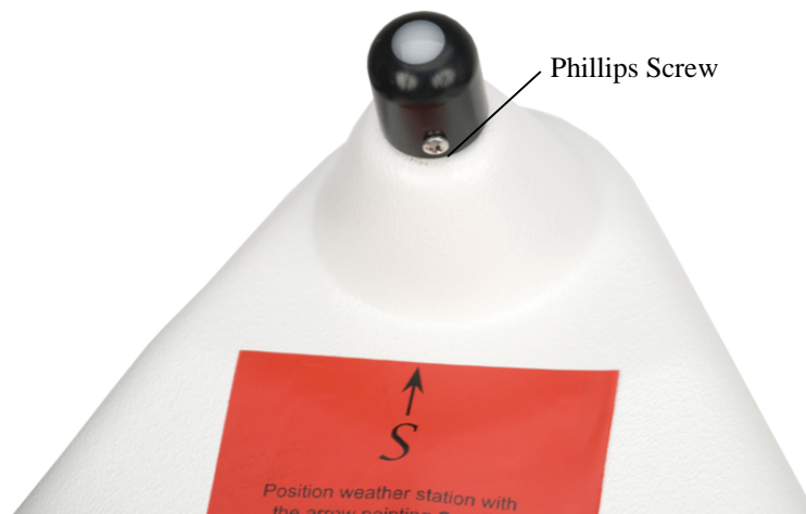
FIGURE 6-4. Solar radiation sensor
