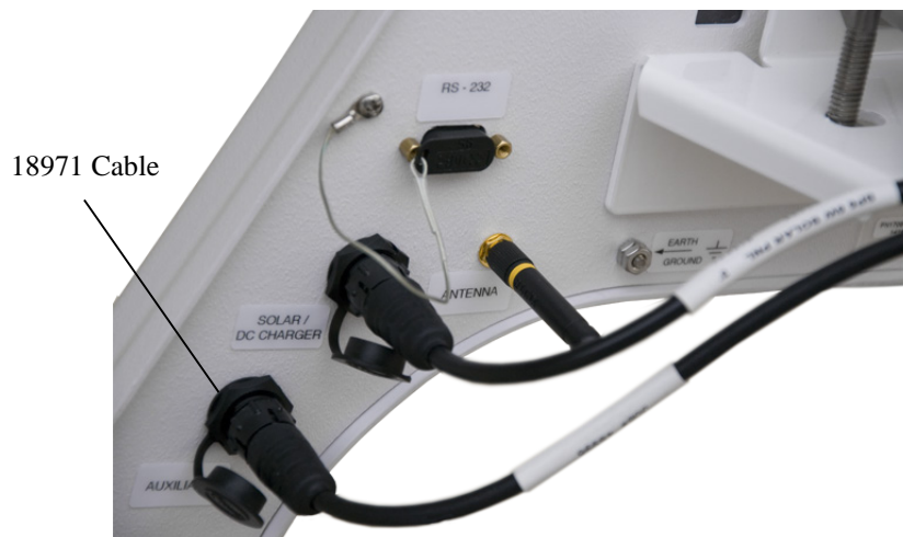
FIGURE 5-22. 18971 cable connected to TurfWeather station
