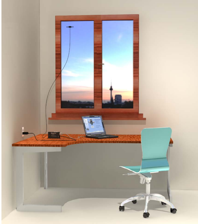
FIGURE 5-15. A typical RF401-series base station
