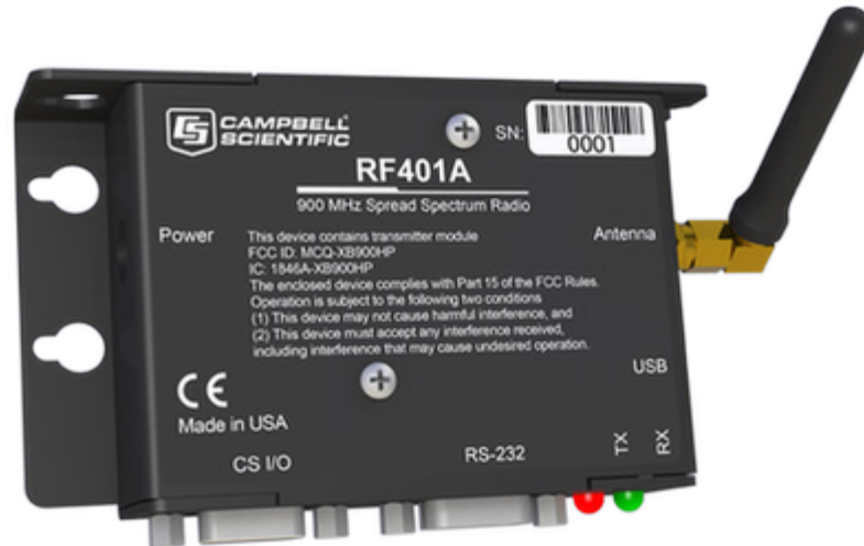
FIGURE 4-6. Radio connections. The serial cable connects to the RS-232 port and the AC adapter connects to the Power port.
