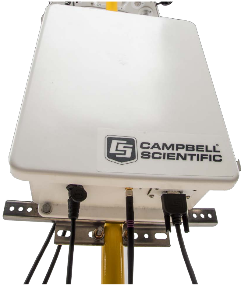
FIGURE 5-26. 18971 cable and 31654 RS-232 cable connected to ATP100 enclosure
