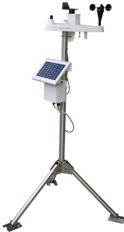
FIGURE 5-16. Short haul enclosure mounted to the 16776 tripod
