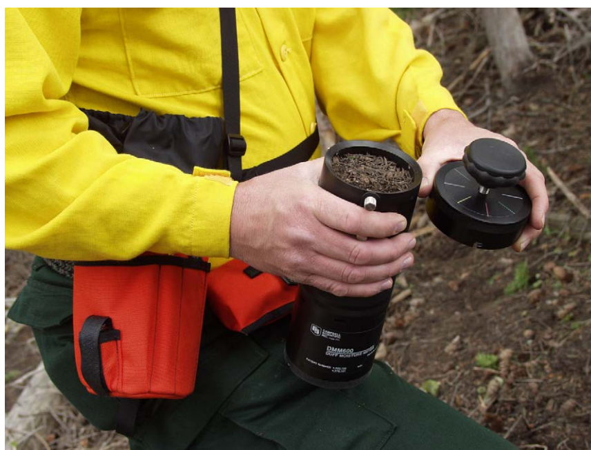
FIGURE 4-3. Duff placed in chamber
