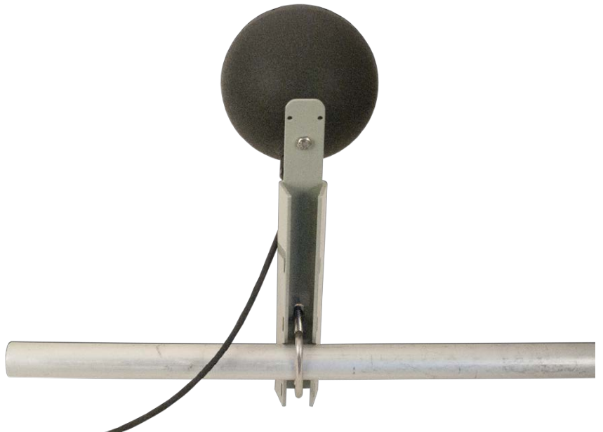
FIGURE 6-5. BlackGlobe mounted to a crossarm (back view)
