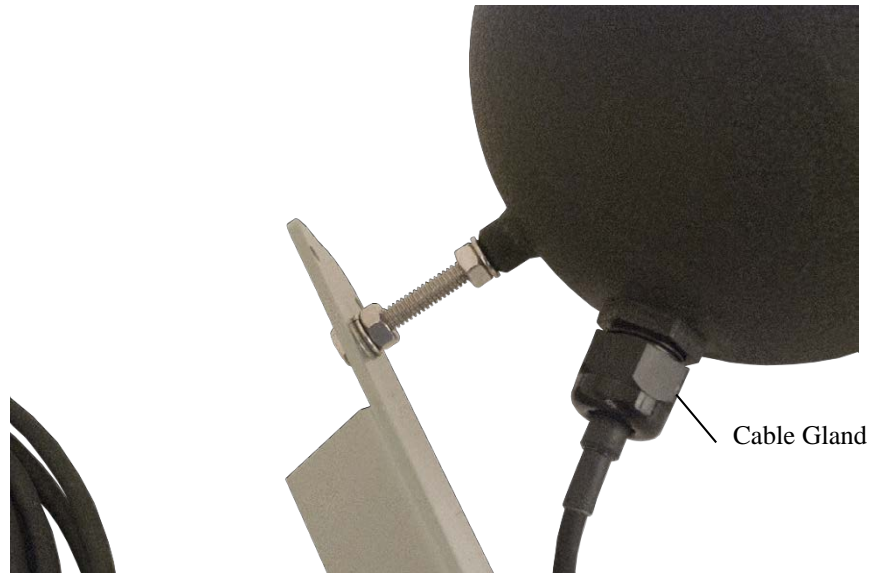
FIGURE 6-3. BlackGlobe fitting and cable alignment
