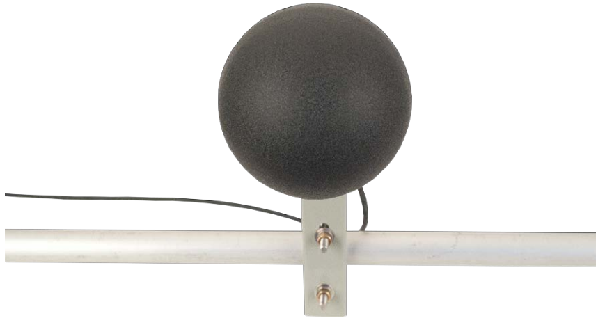
FIGURE 6-4. BlackGlobe mounted to a crossarm (front view)
