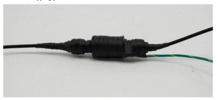
8. Secure the assembly, perhaps to the mast that supports the antenna. UV resistant cable ties are versatile fasteners. Point down the end from which the ground wire emerges to minimize the chance of moisture entry.
