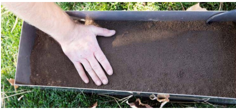
FIGURE 3-3. SoilVUE™10 with 5 cm of soil packed on top of it
