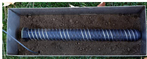
FIGURE 3-1. SoilVUE™10 placed in a trough
