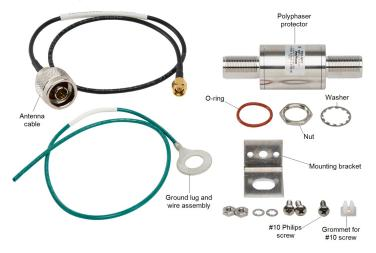
Campbell Scientific surge protector kits protect RF equipment by equalizing the potential difference between the center pin of the coax cable and its shield. The kits include a capacitive-coupled gas tube protector with multi-strike capability. If properly grounded, the capacitor will block low frequency surge currents induced onto the center-pin from the antenna side until the gas tube reaches a high enough voltage to shunt the surge to ground.
