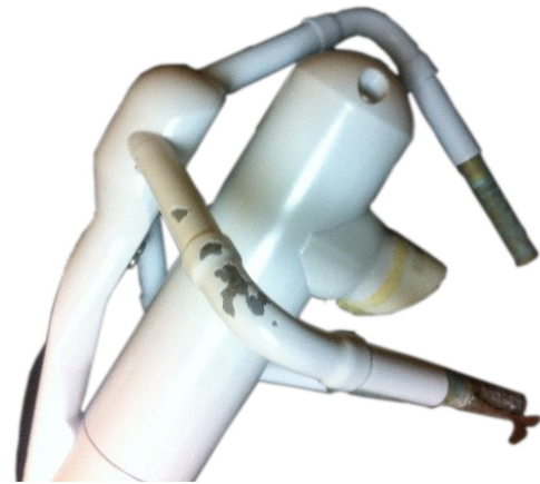
Figure 3. Painting removed where it was apparently impacted on the knuckle of side claw (first sonic path) among the top three sonic transducer claws of the IRGASON sonic anemometer (serial no.: 1131).
