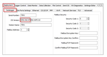
11. Check to see what version of the WiFi daughter board operating system your datalogger is running. As in the previous step, you can see this information in the **Deployment** | **Datalogger** tab in *DevConfig*. The **OS Version** field shows the datalogger operating system version and WiFi daughter board operating system version (in red below) currently loaded into the datalogger.
