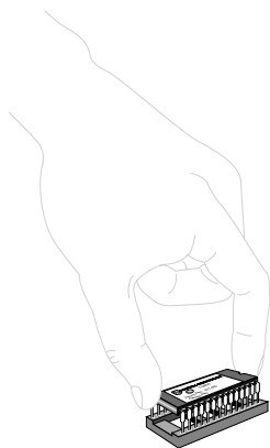
FIGURE 8. Inserting the New PROM
