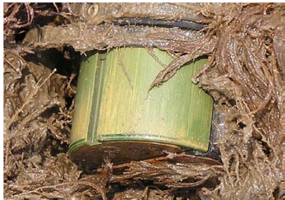
Figure 22. Brass after 137 days at Skidaway
