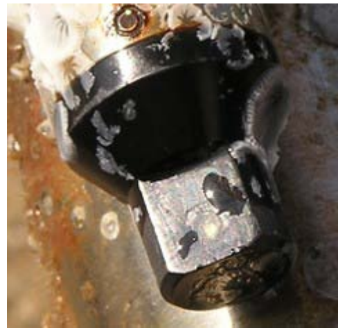
Figure 8. Baseline sensor, day 36 after manual cleaning
