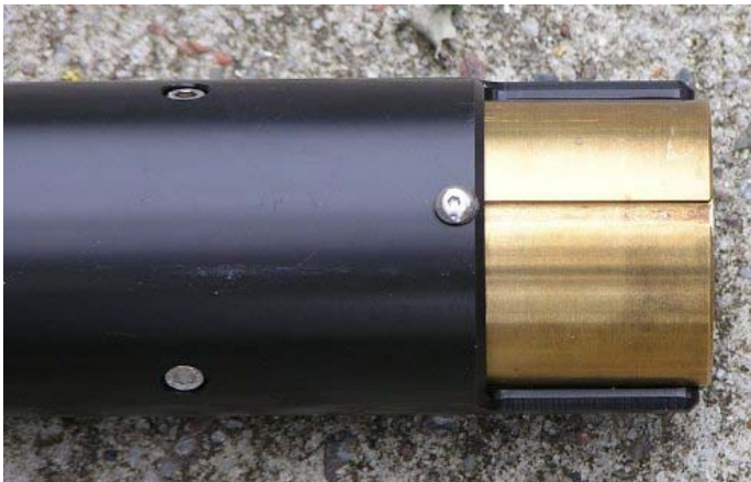
Figure 2. Shutter closed over sensor optics
