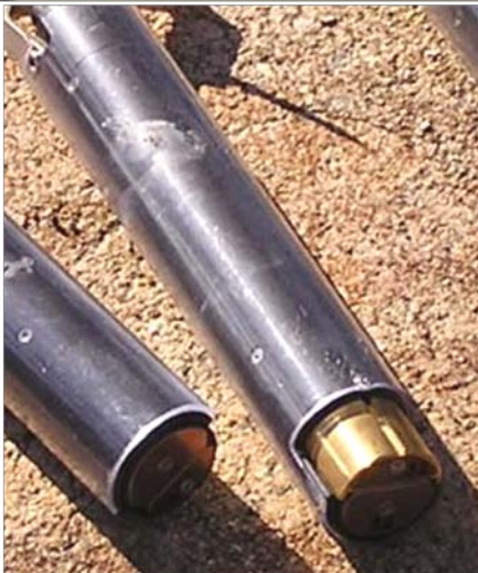
Figure 6. Plastic sleeve provides easy cleaning
