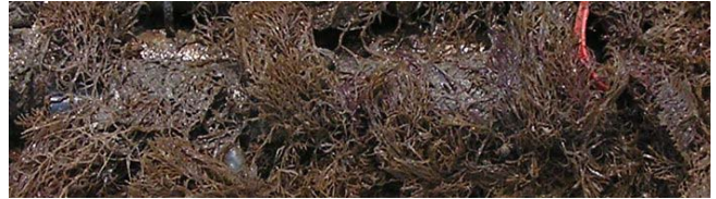
Figure 20. Plastic sleeve after 137 days at Skidaway
