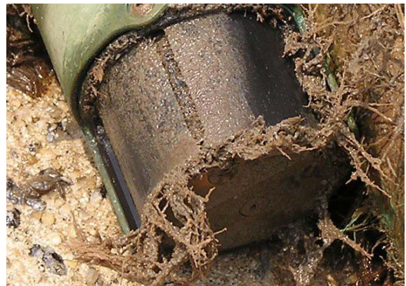
Figure 21. Delrin after 137 days at Skidaway
