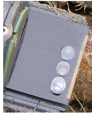
Figure 3. Wiper displaces fouling as it pushes across optics
