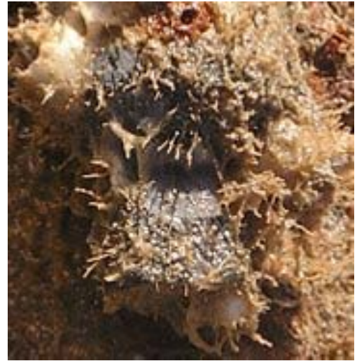
Figure 7. Baseline sensor, day 36 before cleaning
