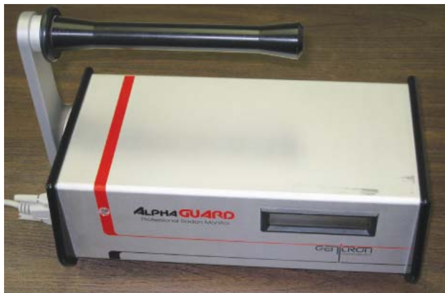
Figure 1. Front view of the AlphaGUARD Professional Radon Monitor Model P30 (standard version).
