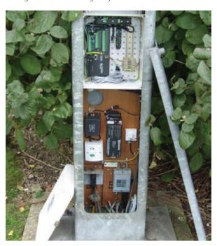
Above shows the instruments used in one of the AWS that monitors the Channel Tunnel.
