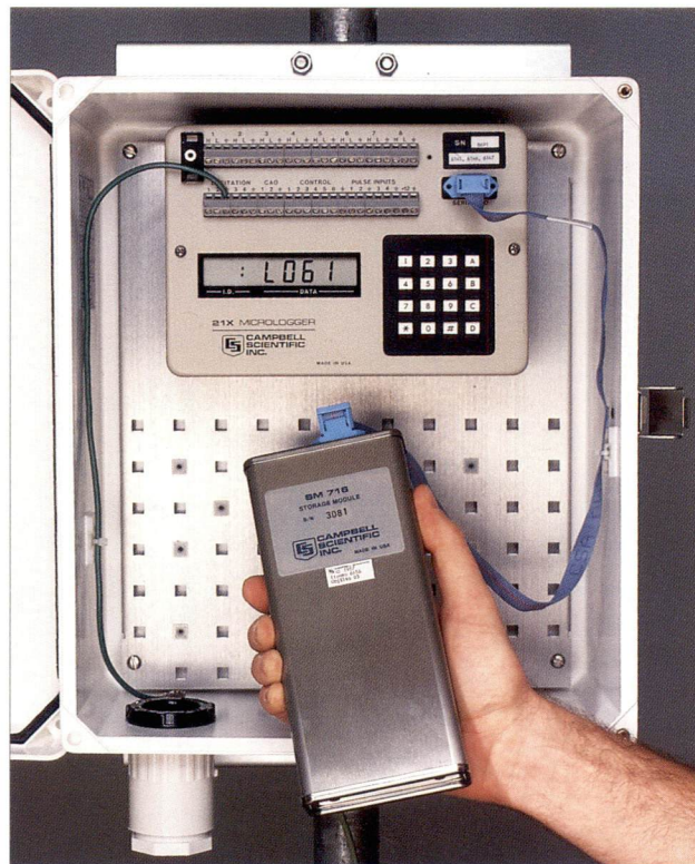
An SM716 stores data from a 21X Micrologger.
