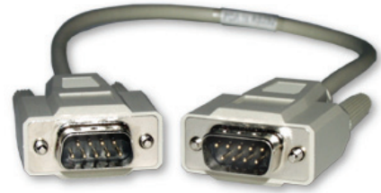
The #18663 null modem cable connects directly to the datalogger's RS-232 port. This cable is the only option available for connecting a Raven110 modem to a CR200-series datalogger.
