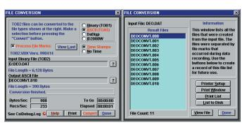
The convert utility converts the datalogger's data into other formats allowing the data to be displayed using other software (e.g., DaDisp spread sheet programs).
