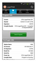
The Collect Data Page (left) is for collecting the datalogger's data. The Status Page (right) displays important information
