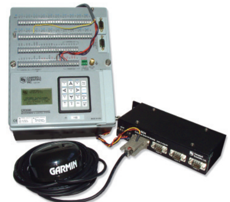
The sensor interfaces with the datalogger via the RJ45 to RS-232 Adapter and an SDM-SIO4 module. This interface option is compatible with our CR800, CR850, CR10X, CR1000, CR3000, CR5000, and CR9000X dataloggers.
