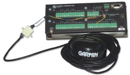
An RJ45 Interface Cable connects the sensor to the datalogger's control ports. This interface option is compatible with our CR800, CR850, CR10X, CR1000, and CR3000 dataloggers.
