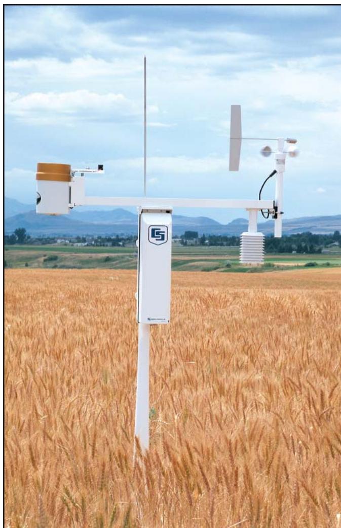
The ET106 provides real-time weather measurements and calculates ET_0 on an hourly and daily basis.
