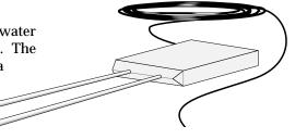
The Water Content Reflectometer consists of two stainless steel rods connected to a printed circuit board. A shielded four-conductor cable is connected to the circuit board to supply power, enable the probe, and monitor the pulse output. The circuit board is encapsulated in epoxy. The probe rods can be inserted from the surface or the probe can be buried at any orientation to the surface.
