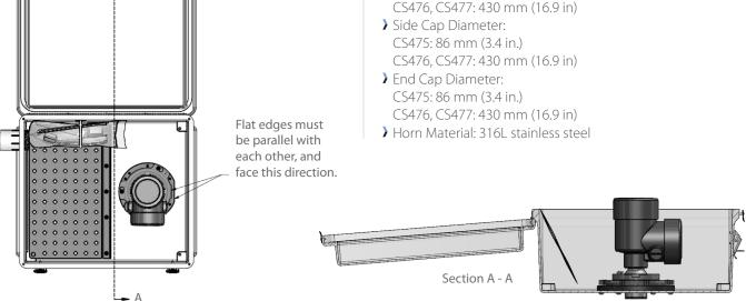
At left is a top view of the field enclosure showing the sensor placement and backplate for mounting a datalogger. At right is a cut away view of the field enclosure showing sensor placement. The horn fastens to the sensor on the outside of the enclosure (not shown).
