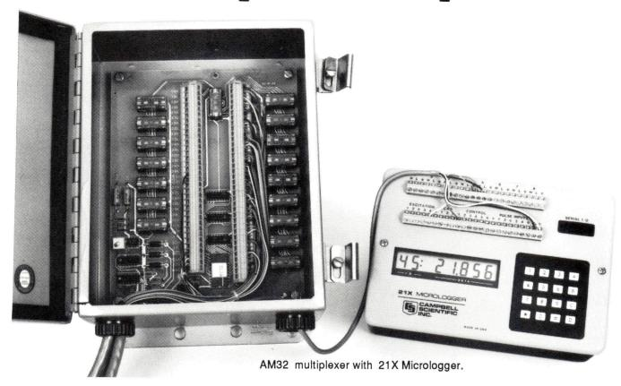
The AM32 Input Multiplexer sequentially connects as many as 32 sensors to a single CR10, CR7(X), or 21X input channel. Many sensor types are compatible with the AM32; examples include thermistors, thermocouples, pyranometers and soil moisture probes. Concurrently scanned sensors may be of a single type or of certain compatible combinations. The AM32 reduces lead wire cost on long wire runs because only 6 leads are required to connect to the datalogger.
