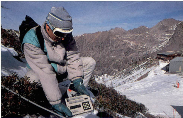
Programs can be entered or edited on-site via the 21X's keyboard and display.
