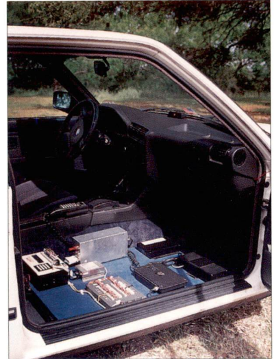
A cross-country vehicle test system records performance data and vehicle position for transmission via cellular phone.
