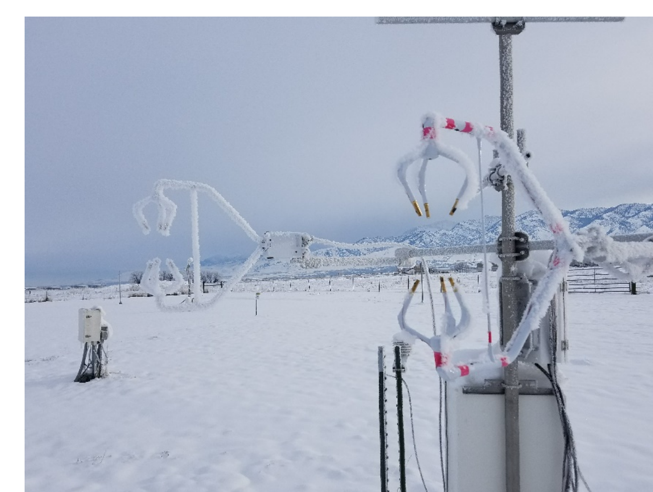
Fig. 3a Heated sonic (right) compared to non-heated sonic (left) during icing conditions
