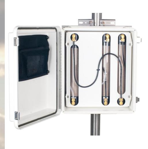
The CPEC200 Scrub Module is an accessory to the CPEC200. It is used to provide a source of zero air for zeroing the EC155 CO<sub>2</sub>/H<sub>2</sub>O analyzer. It uses a small, low-power (2W) diaphragm pump that is mounted in a temperature-controlled and weathertight fiberglass enclosure. Ambient air is drawn through molecular sieve to remove CO<sub>2</sub> and water vapor, and push zero air to the EC155 at approximately 2 l·min<sup>-1</sup> flow.
