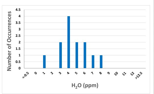
All cylinders tested at  $CO_2 < 0.3$  ppm; below specifications. Water vapor was between 0 and 8 ppm, but still well below practical requirements for an IRGA intended for ambient humidity. In all cases the zero air had equal or less  $CO_2$  and  $H_2O$  after passing through the molecular sieve.
