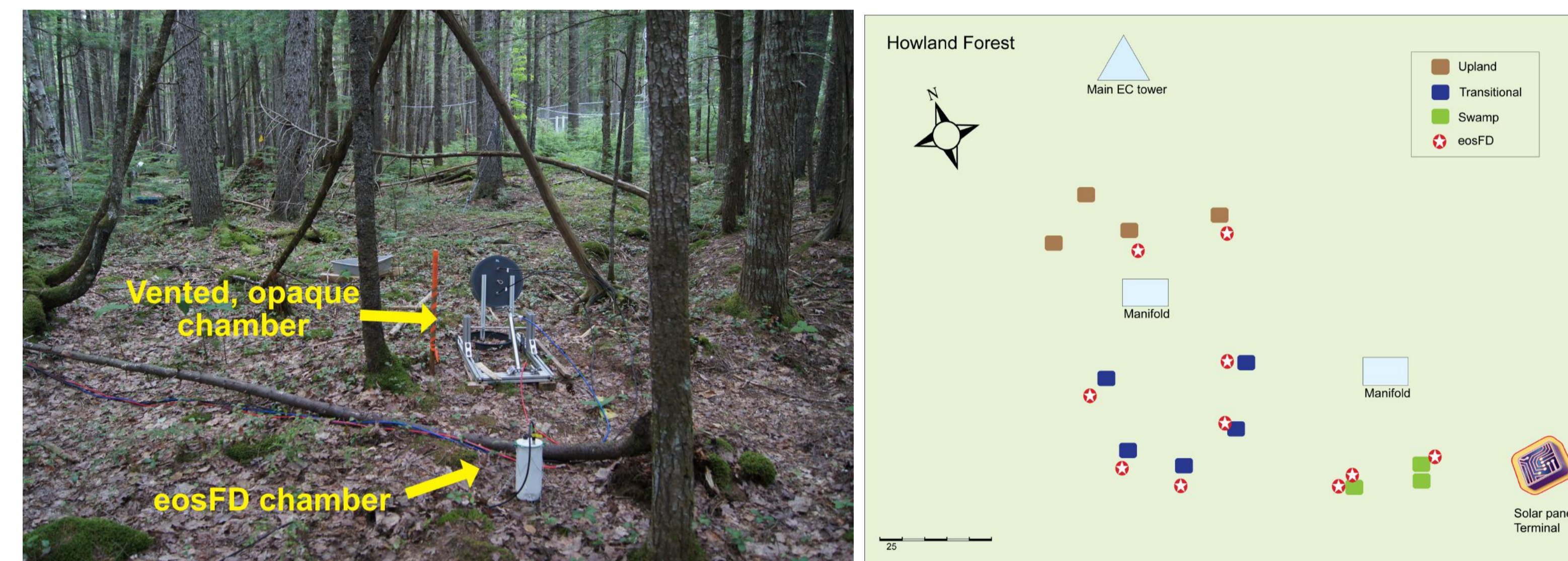
Figure 2: Left - eosFD chamber co-installed at Howland forest alongside an existing automated soil respiration chamber. Right - schematic of the layout of infrastructure at Howland Forest.
