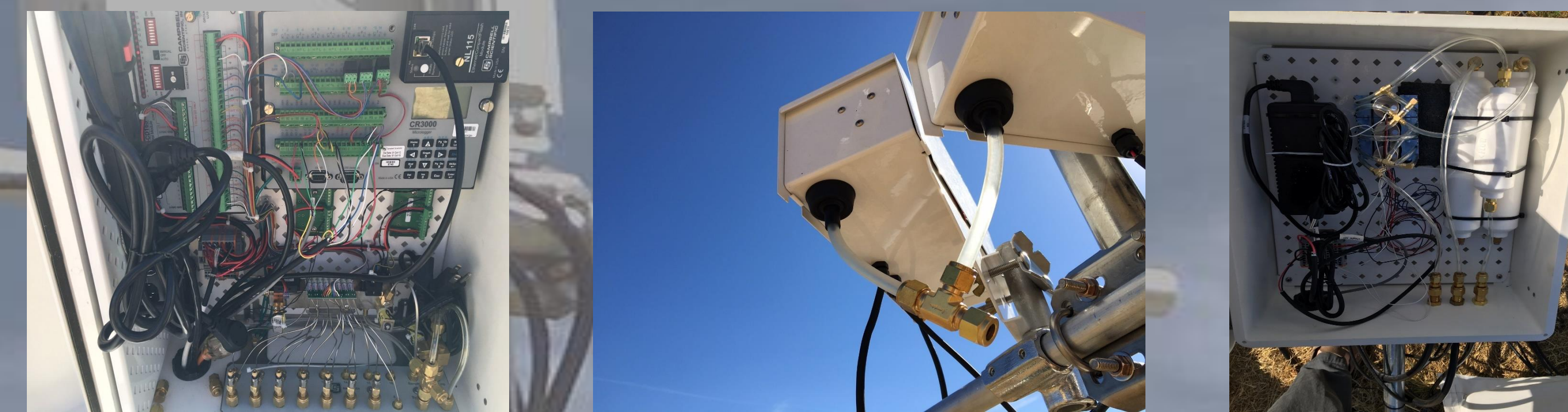
Figure 1: TGA sampling system, AP200 Intakes (in zero-gradient arrangement) and low-power sample and prototype pump module.
