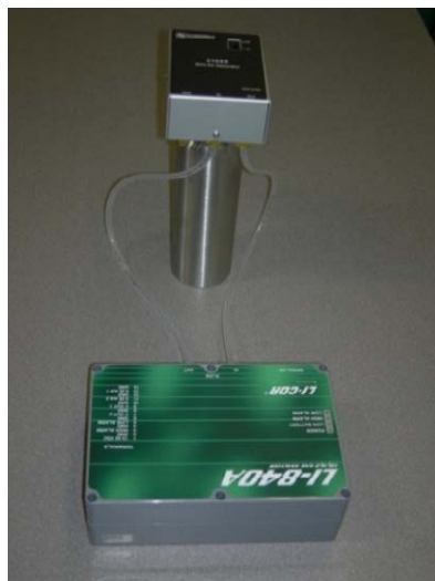
FIGURE 6-5. Zero Air Generator connected to LI-840A
