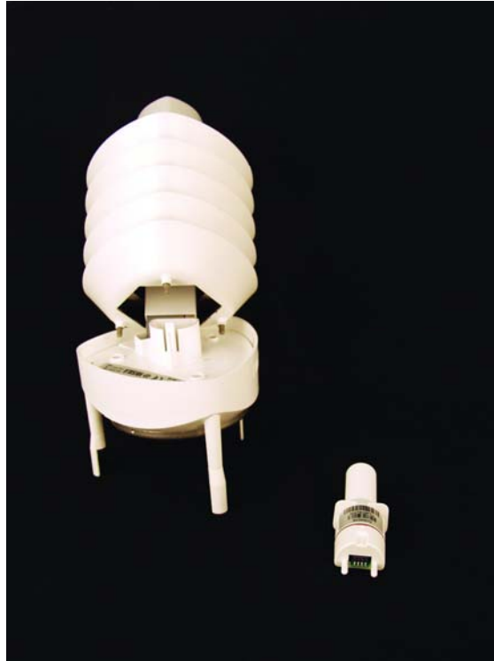
FIGURE 1. Opened WXT510 with the PTU at the right.
