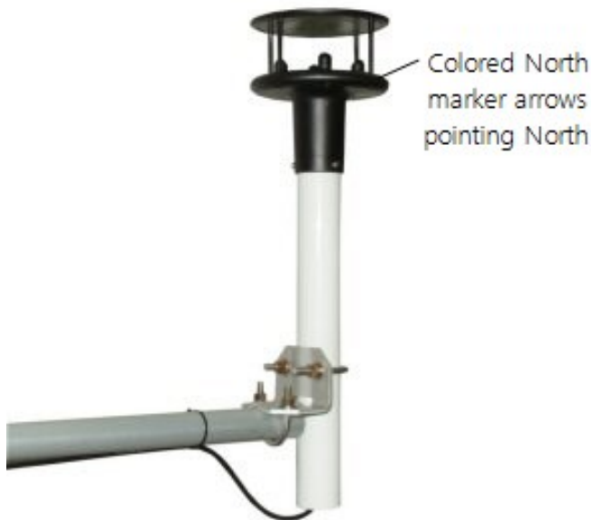
FIGURE 7-1. WindSonic4 mounted on a crossarm
