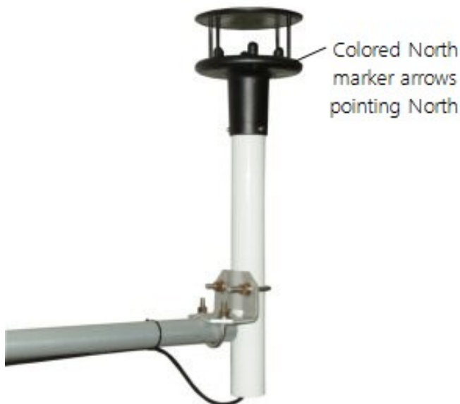
FIGURE 7-1. WindSonic1 mounted on a crossarm
