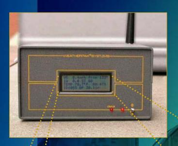
The Receiver/Display is also the interface with the PC and plume dispersion modeling software.
