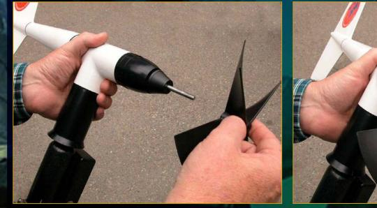
Place the propeller on the front shaft. Either direction is OK.
