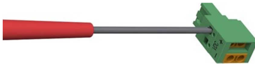
FIGURE 8-3. Opening the power connector terminals
