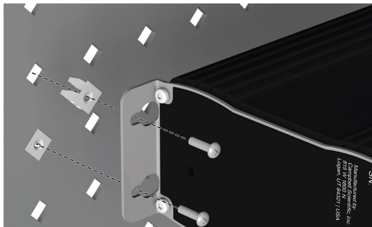
FIGURE 8-4. Enclosure backplate mounting
