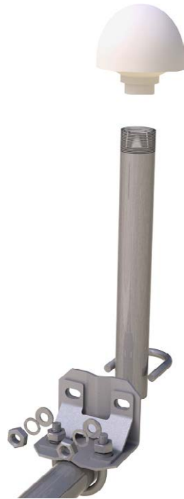
FIGURE 4-5. Exploded view of the GPS antenna mounted to a crossarm via the CM220.
