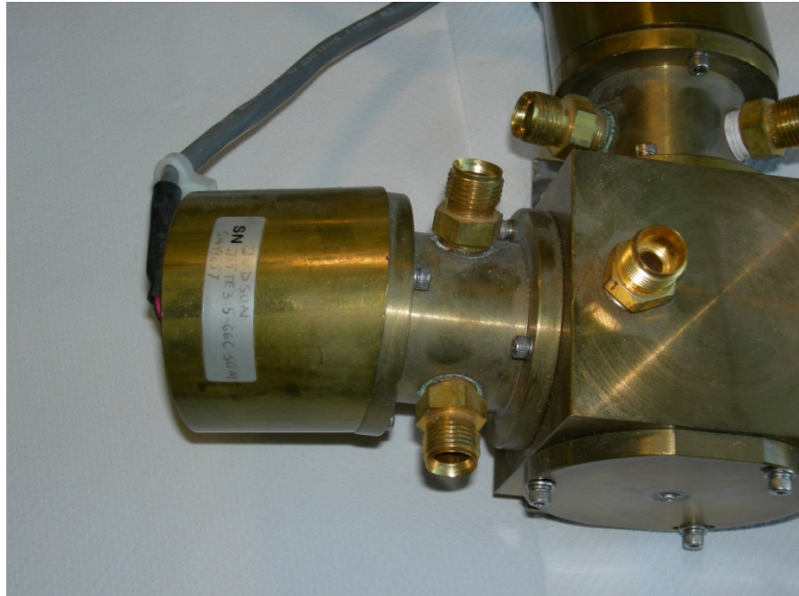
FIGURE H-8. Older style two-piece detector holder and short cell
