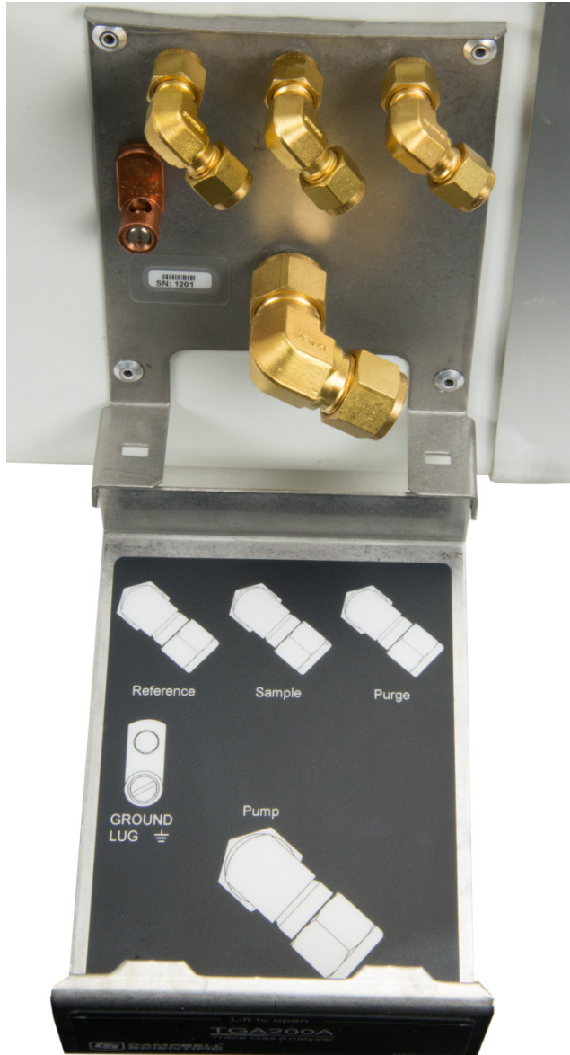
FIGURE 6-10. Plumbing connections located under feedthrough cover of TGA200A
