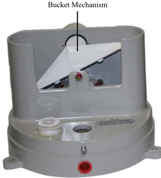
FIGURE 5-1. CS700 Bucket Mechanism (housing not shown)
