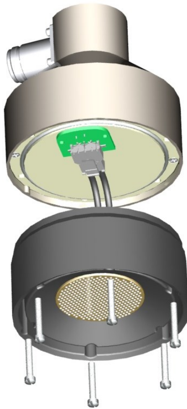
FIGURE 9-3. Remove transducer housing and disconnect wires
