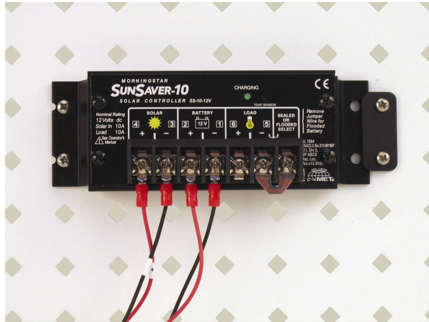
FIGURE 17. Morningstar's SunSaver SS-10-12V Regulator Mounted on an Enclosure Backplate
