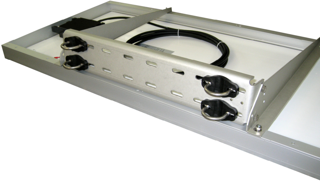
FIGURE 14. Two 5/16-18 x 1.5 U-Bolts are Attached to Each Side of the Solar Panel Mount for Tower Mounting
