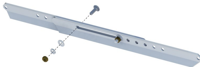
FIGURE 3-10. Assembling the support struts
