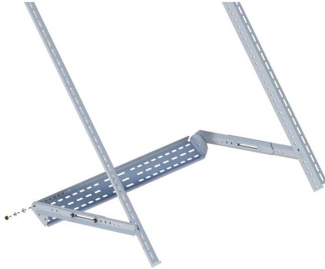
FIGURE 3-12. Attaching the lower mount bracket
