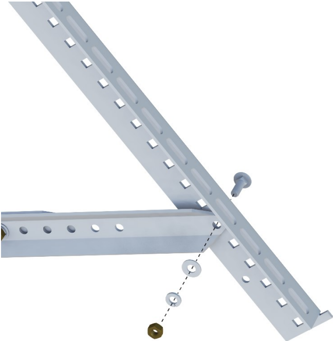
FIGURE 3-11. Attaching the support struts to the mount arms
