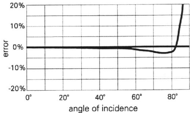
FIGURE 4. Cosine Response of a Typical SP-LITE Pyranometer
