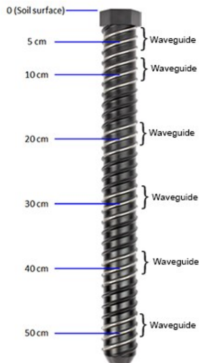
Figure 5-1. SoilVUE 10 waveguides and measurement depths
