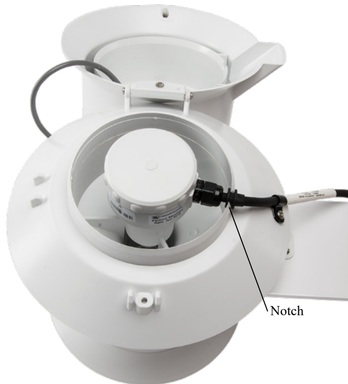
FIGURE 7-4. 43347 probe mounted inside the 43502 shield
