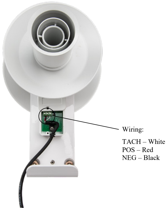
FIGURE 7-5. 43502 shield terminals
