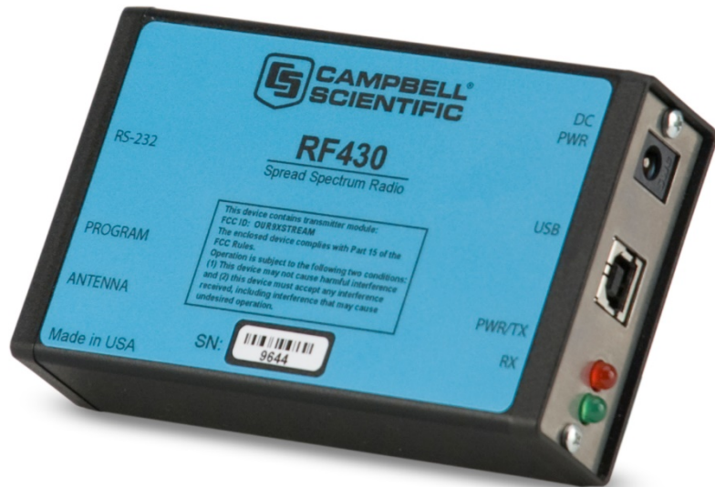
FIGURE 1-2. RF430 has a USB port allowing it to be connected directly to a PC's USB port.
