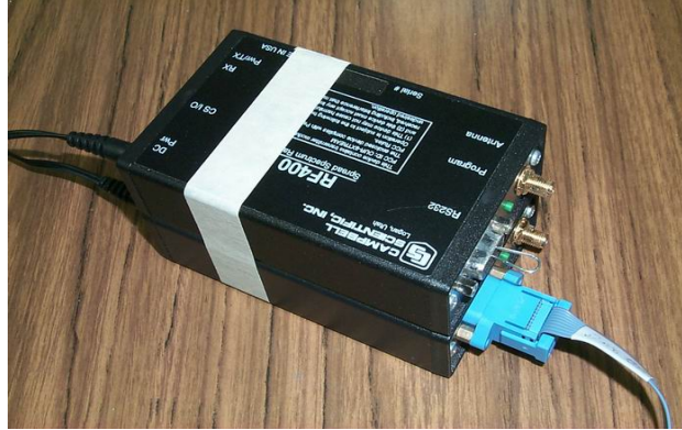
FIGURE K-1. Loop-back Test without Antennas
