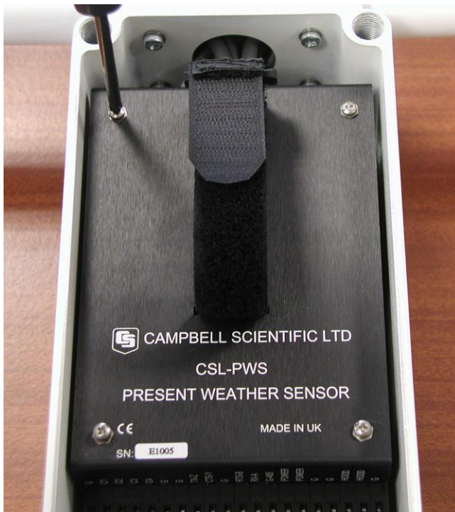
Figure 3-10. Removal of DSP cover
