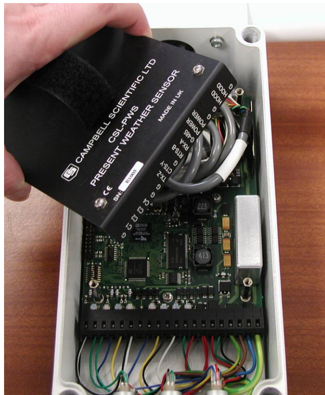
Figure 3-11. Exposing the DSP board
