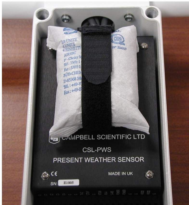
Figure 3-8. Mounting the desiccant pack on the DSP cover
