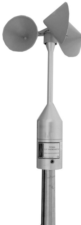
FIGURE 7-1. P2546A wind sensor installed on mounting pipe
