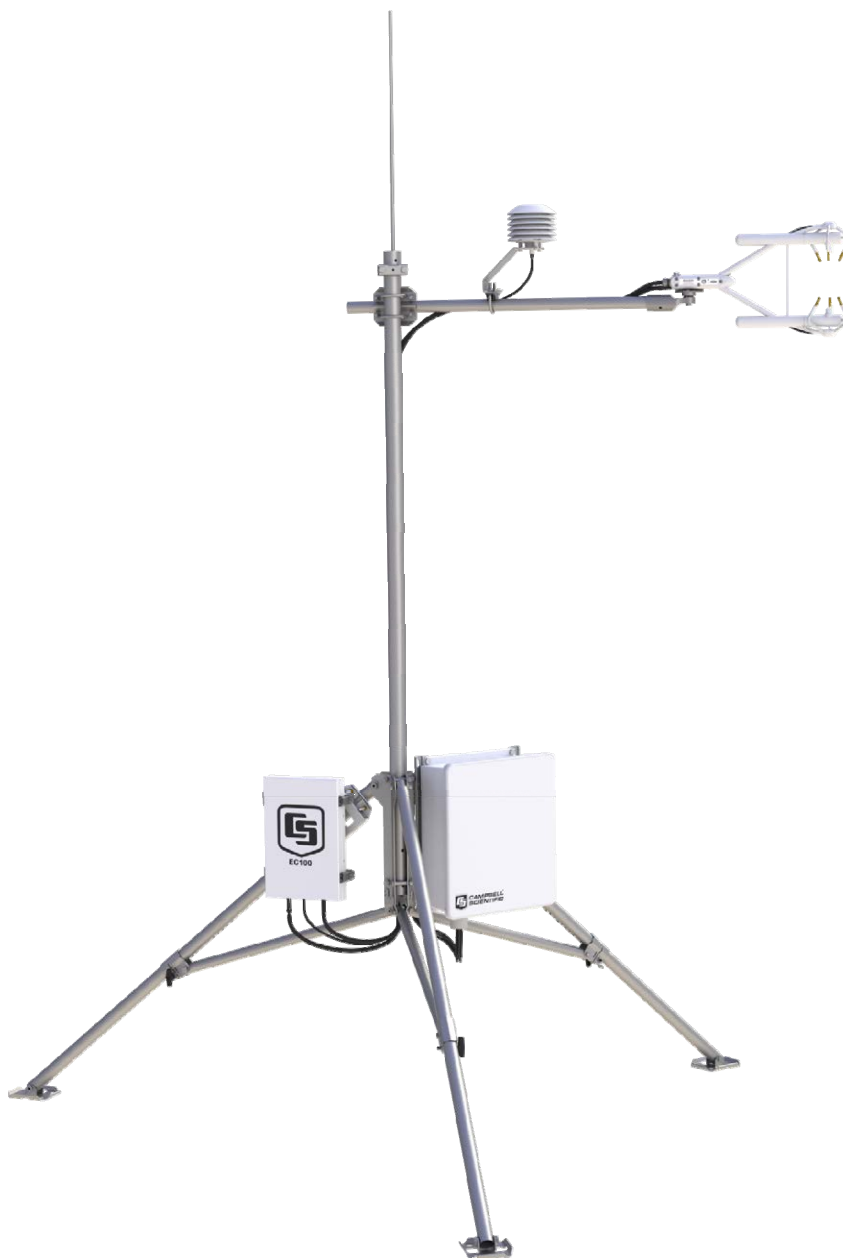
FIGURE 2-1. Open-Path Eddy-Covariance (IRGASON) System
