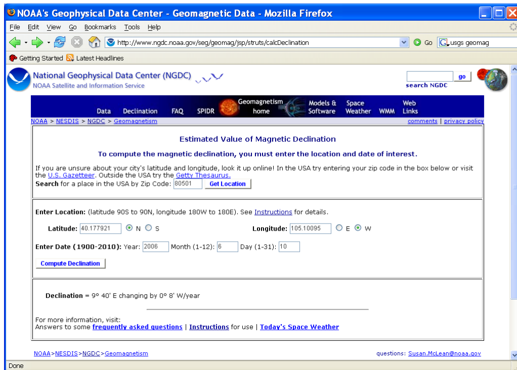
FIGURE A-4. Online magnetic declination calculator with inputs and output for Longmont, CO
