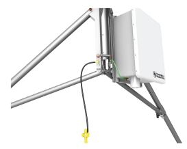
3. Attach the CM20X crossarm to the tripod mast.
