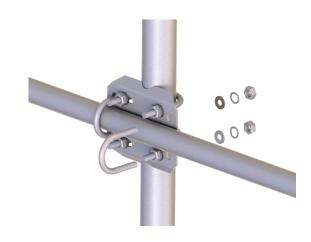
4. Mount the IRGASON or EC150/CSAT3A to the crossarm and point it into the prevailing wind
