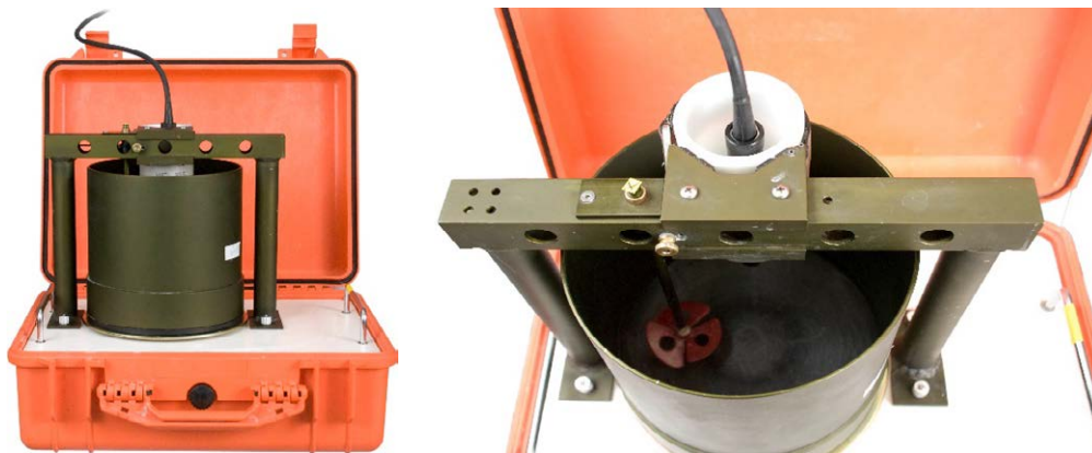
FIGURE 7-8. Portable Sediment Suspender (left) and OBS beam orientation in suspender tub (right)
